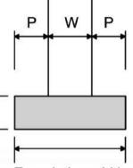
Foundation width should not be less than the appropriate
