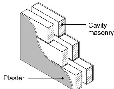
(c) **WT 3** - Cavity masonry with plaster finish
