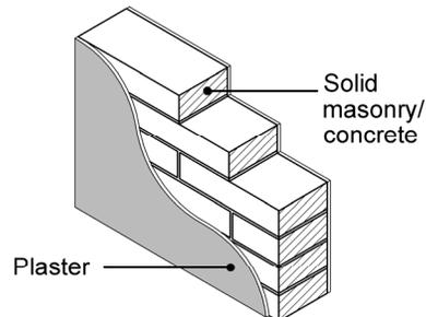
(a) **WT 1** - Solid masonry/ concrete with plaster finish
