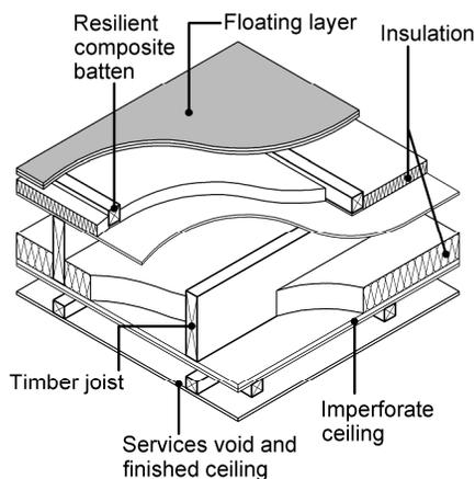
(c) FT 3 Floating layer on timber base with ceiling
