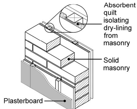
(b) **WT 2** - Solid masonry with dry lining
