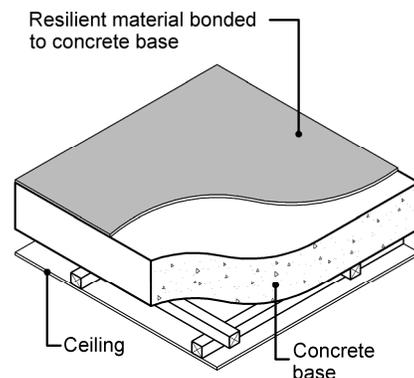
(a) FT 1 Resilient material bonded to concrete base with ceiling
