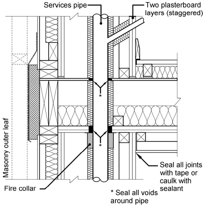
**Services pipes through FT 3 (excluding gas pipes)<sup>1</sup>**
