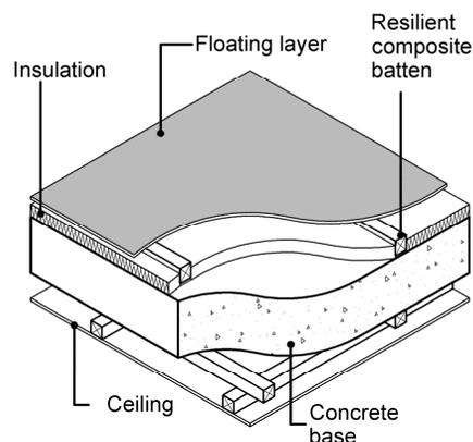
(b) FT 2 Floating layer on concrete base with ceiling
