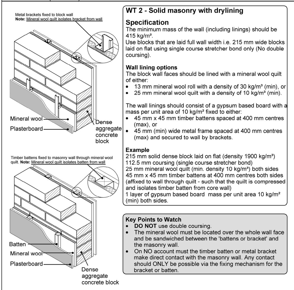
**Diagram 9 WT 2 Solid masonry with dry lining – Flanking requirements at an external (flanking) wall**
