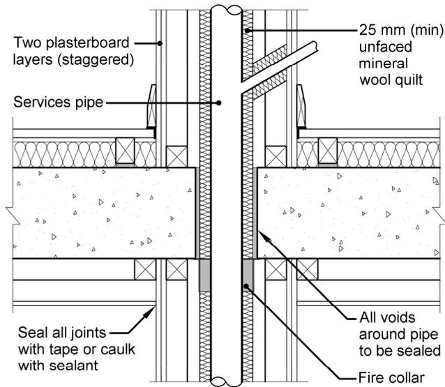
**Services pipes through FT 2 (excluding gas pipes)<sup>1</sup>**
